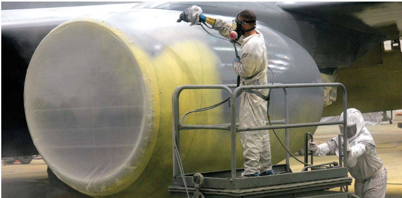
A painter at Tinker Air Force Base puts the first coat on a KC-135 Stratotanker engine cowling.
